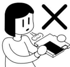
Do not blow into the Game Pak. It is not a harmonica. To fix a blank or scrambled screen, turn the power off and remove and reinsert the Game Pak. If that does not work, clean the edge connector with a cotton swab soaked in isopropyl rubbing alcohol and let it fully dry.
